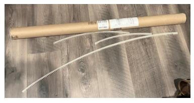
Gears Arrived 20240113 1 tooth per cm(~26 teeth in 10") by 0.5" wide 0.2" tooth depth
